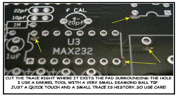
The first pair of trace cuts is where the +5 volt power trace leaves the MAX232 chip, on Pin 16 and enters the OSC CAN socket on Pin 14. Form the picture above, you can see the grind marks where I ground off the small trace just as it exits the actual solder pad.
