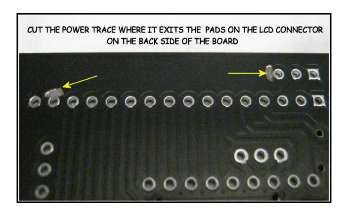
Likewise, the +5 volt power trace from the contrast pot to the LCD backlight pad is shorted to the ground plane on the bottom side of the circuit board. Cut the 2 traces just before they enter the ground plane and solder in a short piece of hookup wire to connect the two pads together.
